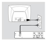
After everything is connected properly, plug in the AC power cord to the power outlet. Never make or change any connections with the power switched on.
