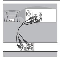
Use the composite video cable (yellow) to connect the DVD player's VIDEO(CVBS) jack to the video input jack(or labelled as A/V in,Video In or Composite) on the TV(cable supplied). To hear the sound of this DVD player through your TV, use the audio cables(white/red)to connect AUDIO OUT(L/R)jacks of the DVD player to corresponding AUDIO IN jacks on the TV(cable supplied).
