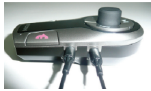
Line in & Line out
