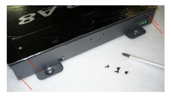
2) For the next step you'll need a large flat screwdriver and a hammer to open the pre-punched connector mounting holes.
