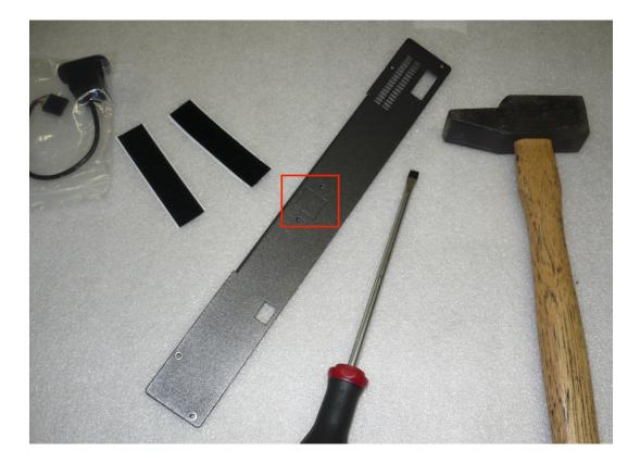
3) Place the screw-driver as pictured and break the lower attachment using the hammer.
