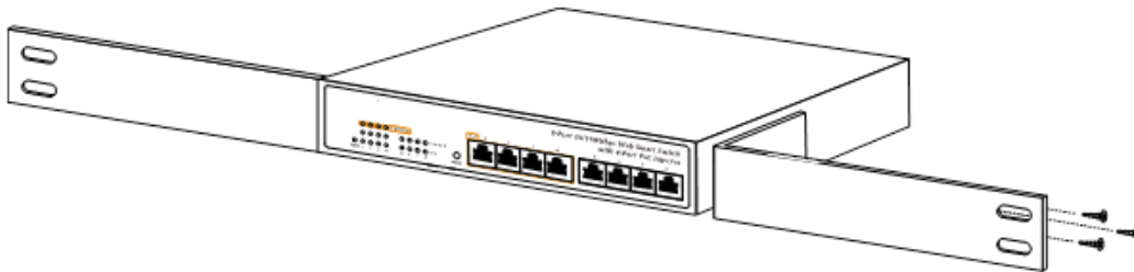
Figure 2-4 Attaching the brackets to the Switch.
