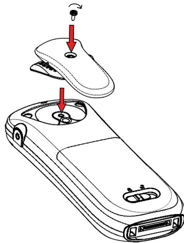
Figure 10. Screw the hinge-type clip into position.
