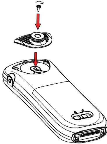
Figure 11. Screw the swivel-type clip into position.
