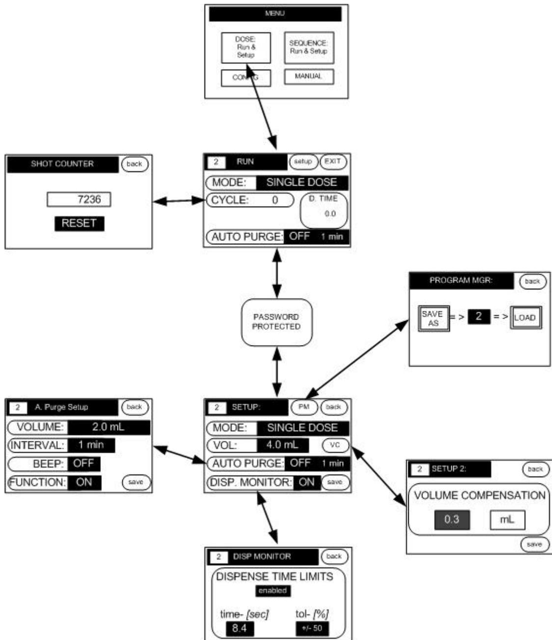
1. The RUN Screen comes into view during normal operation. A number at the top left corner of the screen indicates the program the machine is currently running. The active program will be the last program the machine was running. This screen gives access to the setup screen. Touch the Dose box to reset the cycles counter.
