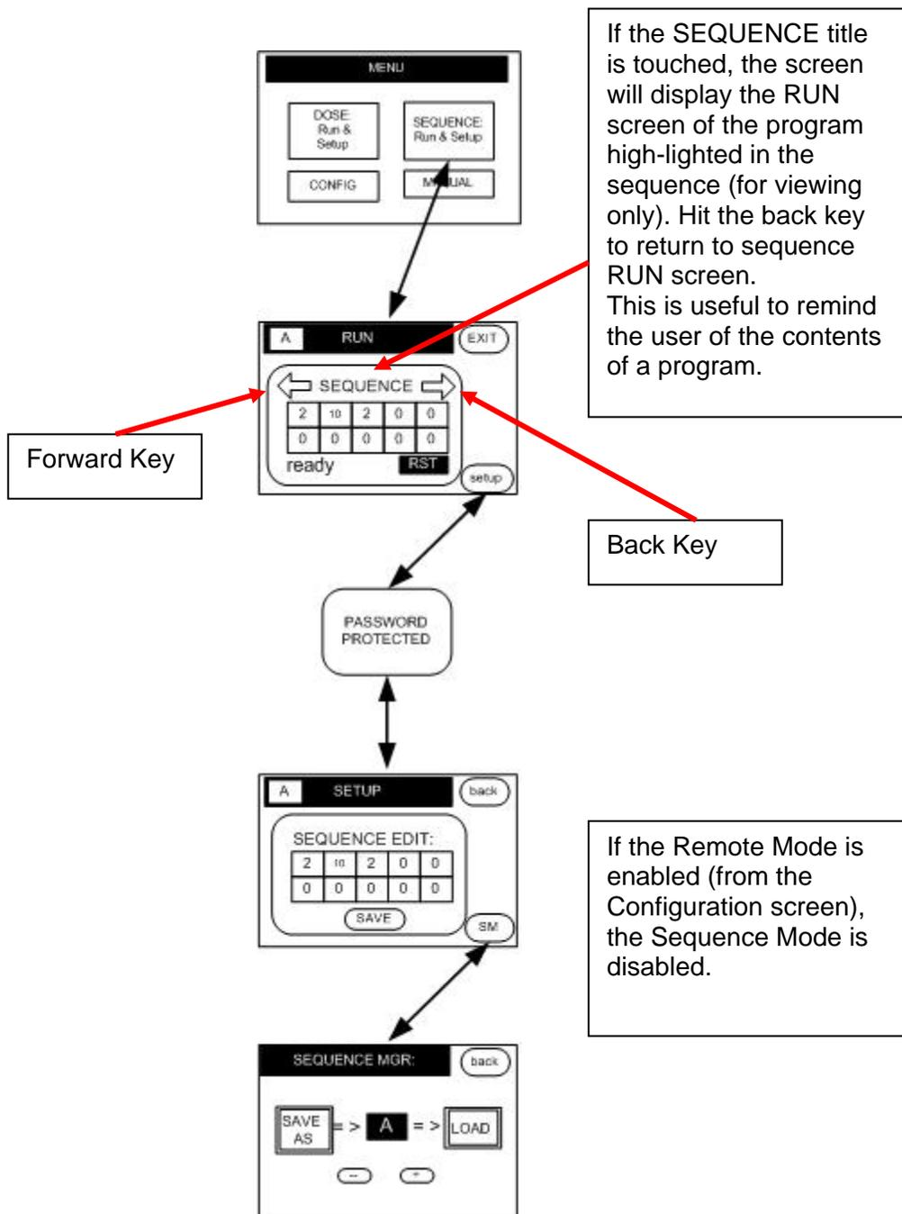
7. SEQUENCE SETUP allows a (serial) sequence of programs to be loaded in up to 10 positions. A zero is seen as a reset (back to the start of the sequence).
