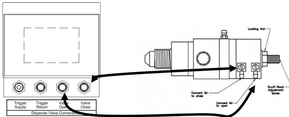
6. To pneumatically cycle the machine, place an air pulse on the Trigger Return port at the Dispense Valve Connections.
