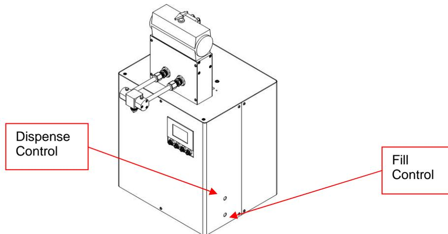
8. Adjust the pumps Fill (re-charge) rate by adjusting the bottom flow control on the main actuator (CW for slower; CCW for faster); accessible via panel holes on the right side of the machine.
