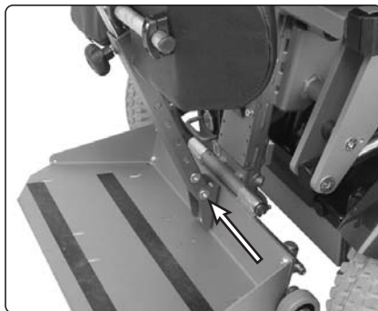
The knee support is mounted with one screw.
