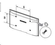
Remove the screws in the mounting holes before you install the wall mount.
