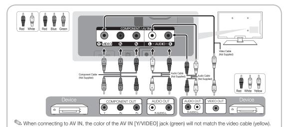
Tor better picture quality, the Component connection is recommended over the A/V connection.
