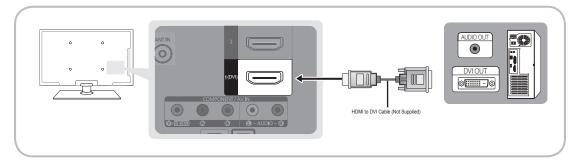
When connecting a HDMI to DVI cable, the Audio cable could not connect.
