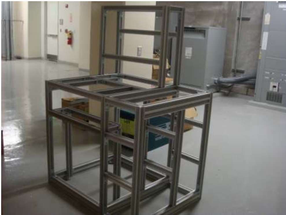
Figure 4.1. Frame used to build the PECVD machine.
