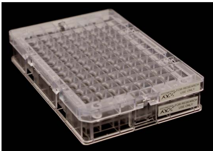
Figure 5.21 Array Plate Hyb Sandwich
