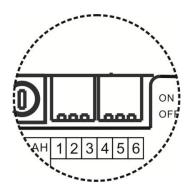
Through the dip switch of 4-5, you can configure the premium low voltage protection level for your system. Following please find data
