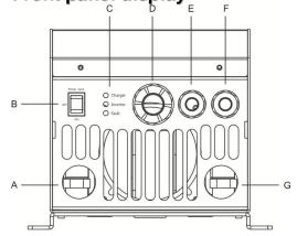
Three LED indicating working mode and fault.
