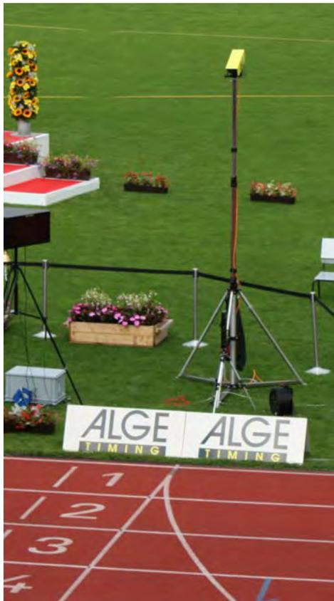
If you use the OPTIc2 with a **Tripod F-STATIV6** with a height of 3.66 m for the camera, you should use a wide angle lens for a track with 8 lanes. Otherwise you do not cover all 8 lanes or you are too far away and have a very flat angle with the runners not being captured completely.
