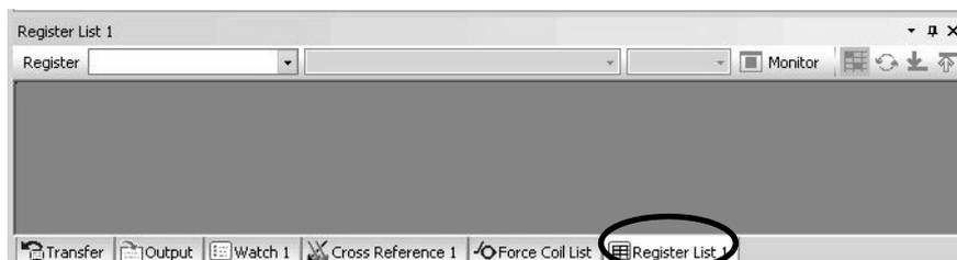
2. Enter the leading register number of the system register “MWxxxxx” (or “DWxxxxx”) to be accessed in the **Register** input field and press the **ENTER** key. The contents of the system register will be displayed starting from the leading register number.
