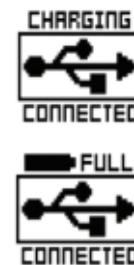
To recharge the battery, attach the 4-pin end of the USB cable to the receptors and connect to your computer. The screens to the left indicate the connection and battery status.
