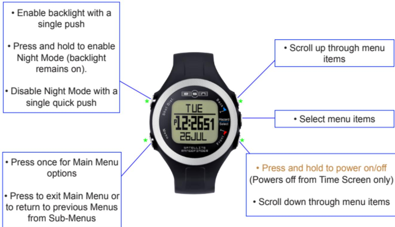
\* Press and hold all four "corner" buttons to perform a hardware reset. This will reboot the watch and restore all default settings. Time will be reset to 12:00 pm when a hardware reset is performed.
