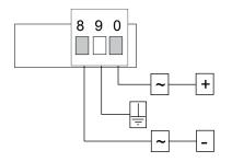
Earth connection - Although a terminal is offered for earth connection, the connection is optional. The instrument does not need this connection for correct functioning nor for compliance with the security regulations.
