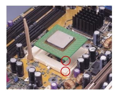
E. Secure the CPU into the socket by pushing the socket lever all the way down. You will hear a click indicating that the lever is in place.
