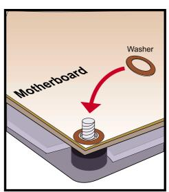
**IMPORTANT:** This step is a MUST! The washers are necessary to prevent shorting.
