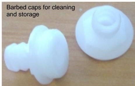
The SBE 16plus is shipped with a kit for cell filling and storage. The kit includes a syringe and tubing assembly, and two anti-foul caps with hose barbs. The tubing cannot attach to an anti-foul cap that is not barbed.
