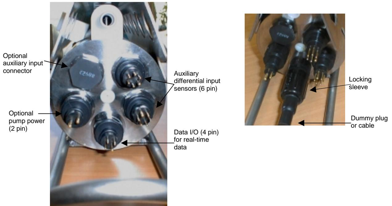
2. Connect the other end of the cables installed in Step 1 to the appropriate sensors.
