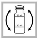
12. Cap the sample cell and invert to mix the extracts. The final volume will be about 25 mL due to the slight solubility of chloroform in water.
