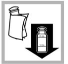
**14.** Wipe the blank and insert it into the cell holder.
