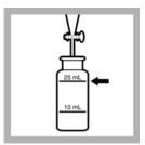
10. Prepared Sample: When the timer expires, wait for the layers to separate. Insert a pea-sized cotton plug into the delivery tube of the funnel. Remove the stopper and drain the chloroform layer (bottom layer) into a sample cell.
