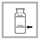
**13. Blank Preparation:** Fill a second sample cell with 10 mL of chloroform.
