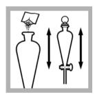
5. When the timer expires, add the contents of one Nickel 2 Reagent Powder Pillow to the funnel. Stopper and invert to mix.
