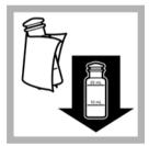
**16.** Wipe the prepared sample and insert it into the cell holder.
