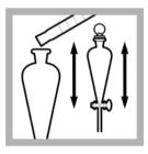
7. When the timer expires, add 10 mL of chloroform. Insert the stopper and invert gently. With the funnel inverted and the tip pointed away from people, open the stopcock to vent.
