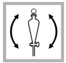
11. Repeat steps 7 through 10 two additional times with 10-mL volumes of chloroform. The five-minute reaction period is not necessary.
