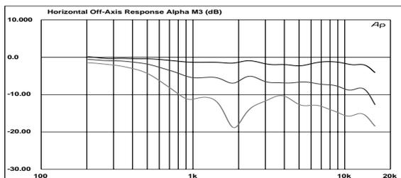
• Figure 11: Horizontal Off-Axis Frequency Response @ 10, 20 & 30°
