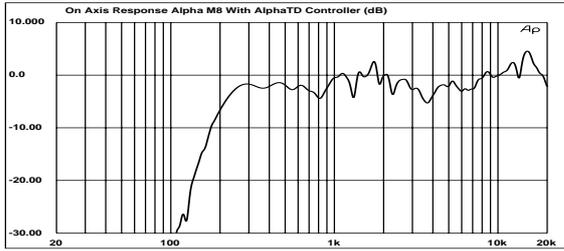
• Figure 13: Frequency Response with Alpha TDcontroller (dB)
