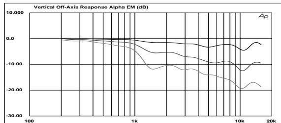
• Figure 24: Vertical Off-Axis Frequency Response @ 10, 20 & 30°
