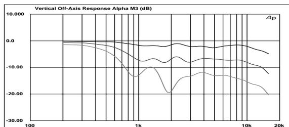
• Figure 12: Vertical Off-Axis Frequency Response @ 10, 20 & 30°
