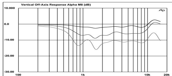
• Figure 18: Vertical Off-Axis Frequency Response @ 10, 20 & 30°
