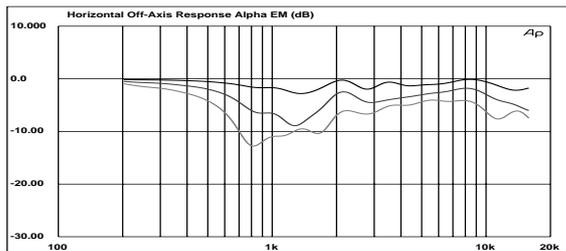
• Figure 23: Horizontal Off-Axis Frequency Response @ 10, 20 & 30°
