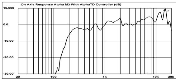
• Figure 7: Frequency Response with Alpha TDcontroller (dB)
