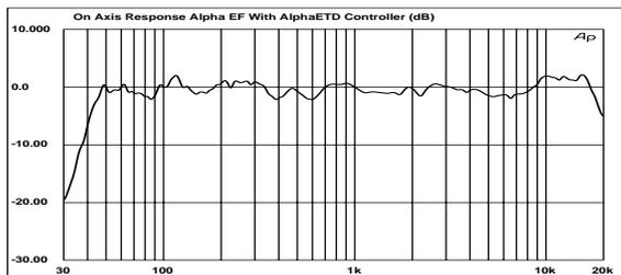
• Figure 25: Frequency Response with AlphaE TDcontroller (dB)
