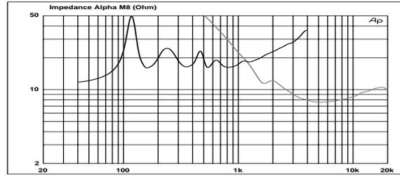
• Figure 14: Impedance (Ohms). *Black: MF, Grey: HF*
