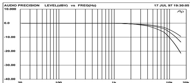
Air absorption over a 50m distance; t=10°C-20°C-30°C
