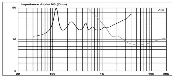
• Figure 8: Impedance (Ohms) *Black: MF, Grey: HF*
