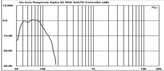
• Figure 1: Frequency Response with Sub TDcontroller (dB)
