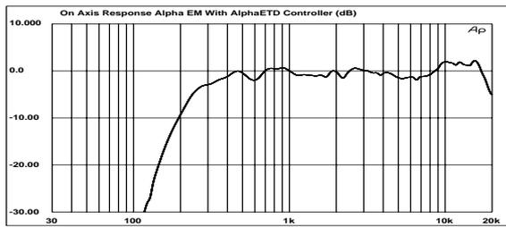
• Figure 19: Frequency Response with AlphaE TDcontroller (dB)
