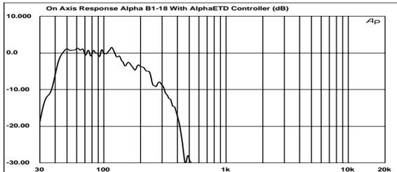
• Figure 3: Frequency Response with AlphaE TDcontroller (dB)
