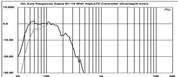
• Figure 5: Frequency Response with Alpha TDcontroller (dB)
