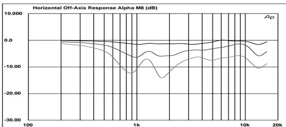
• Figure 17: Horizontal Off-Axis Frequency Response @ 10, 20 & 30°
