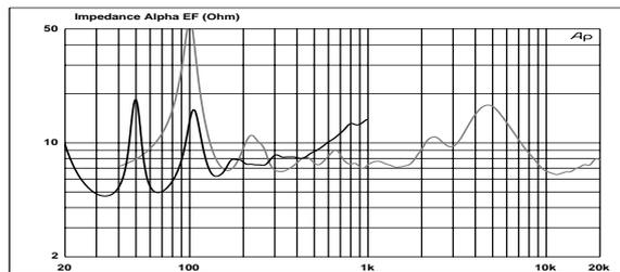
• Figure 26: Impedance (Ohms). *Black: LF, Grey: MF+HF*
