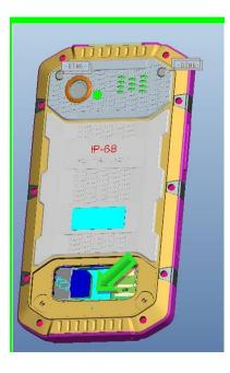
**3.** Open T-Flash card holder and insert T-Flash card into the slot, then close T-Flash card holder as shown in Jig-3
