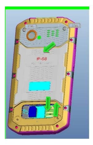
**4. Insert the back cover**: Insert the back cover and rotate four screws clockwise to lock the back cover as shown in Jig-4
