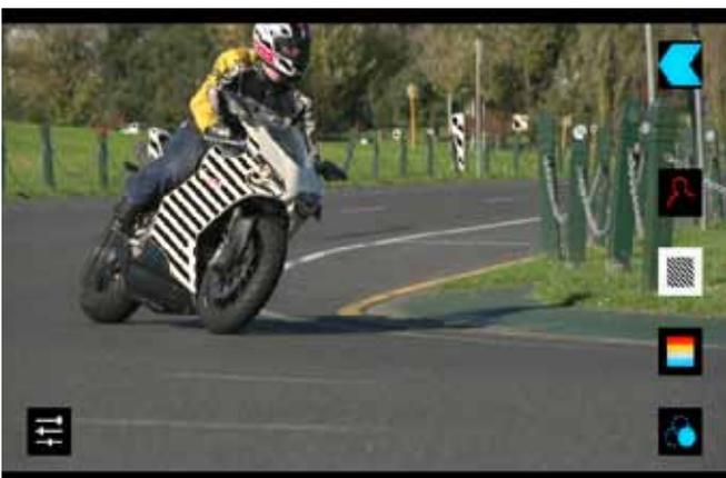
Zebra lines show the parts of the image that are over exposed relevant to the % level set. 95% is usually used for objects, windows and surfaces. 75% is used for checking over exposure of human faces this will indicate reflective or shiny areas on the face.
