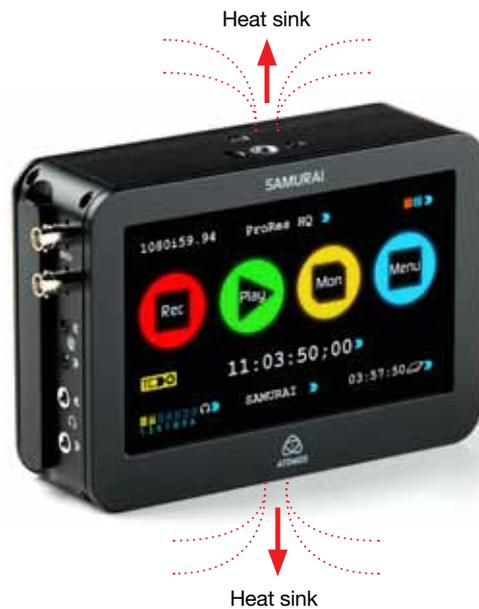
**Do not be alarmed if the top and bottom surfaces seem hot to touch. This is normal part of the design, and shows that your Samurai is dissipating heat successfully.**
