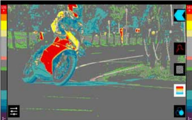
False Colour assigns different colors to areas of different exposure in the image. Instead of just showing what parts of the image are overexposed, it gives a more complete picture of what is going on in the image by using a range of exposure values. Generally speaking, overexposed elements will display as red, and underexposed elements will display as blue.
