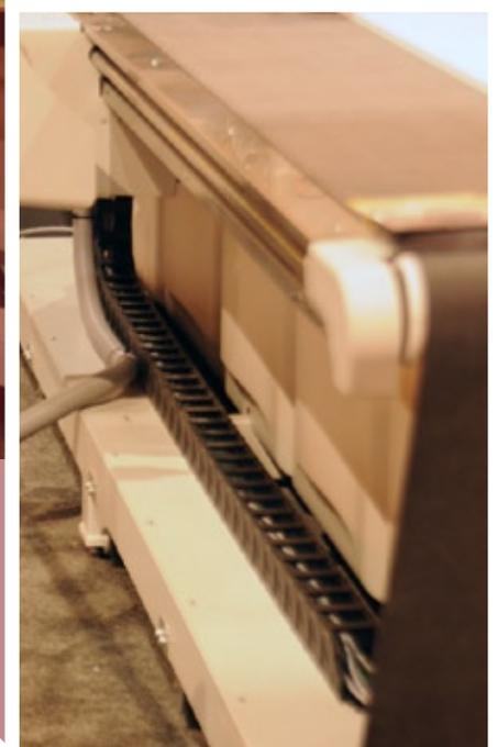
The energy chain is the plastic linked system that holds all the cables and ink tubing so that it does not get rubbed while being moved back and forth to feed the carriage.
