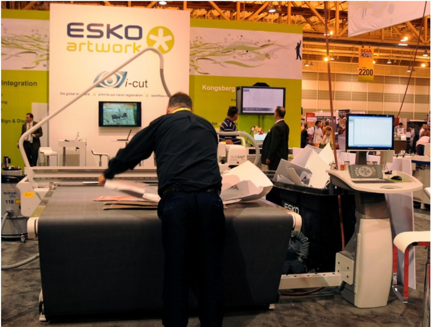
*Maintenance is limited to the inspection and cleaning of the table surface, guideway, rollers, racks, pressure reduction valve, base and the surrounding area; The table surface should be kept clean at all times. For cleaning, use iso-propyl alcohol, use a vacuum cleaner to keep the inside of the conveyor belt clean.*
