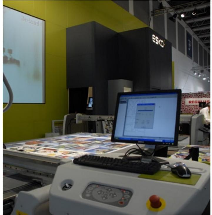
The operational area has a keyboard, a regular computer monitor (about 15 or 16"), and a control pad area with a usual set of buttons to make various selections.
