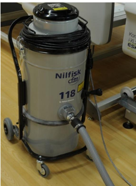
*The waste container should keep clean and do not leave the machine running if is full, because might cause damage to the machine.*
