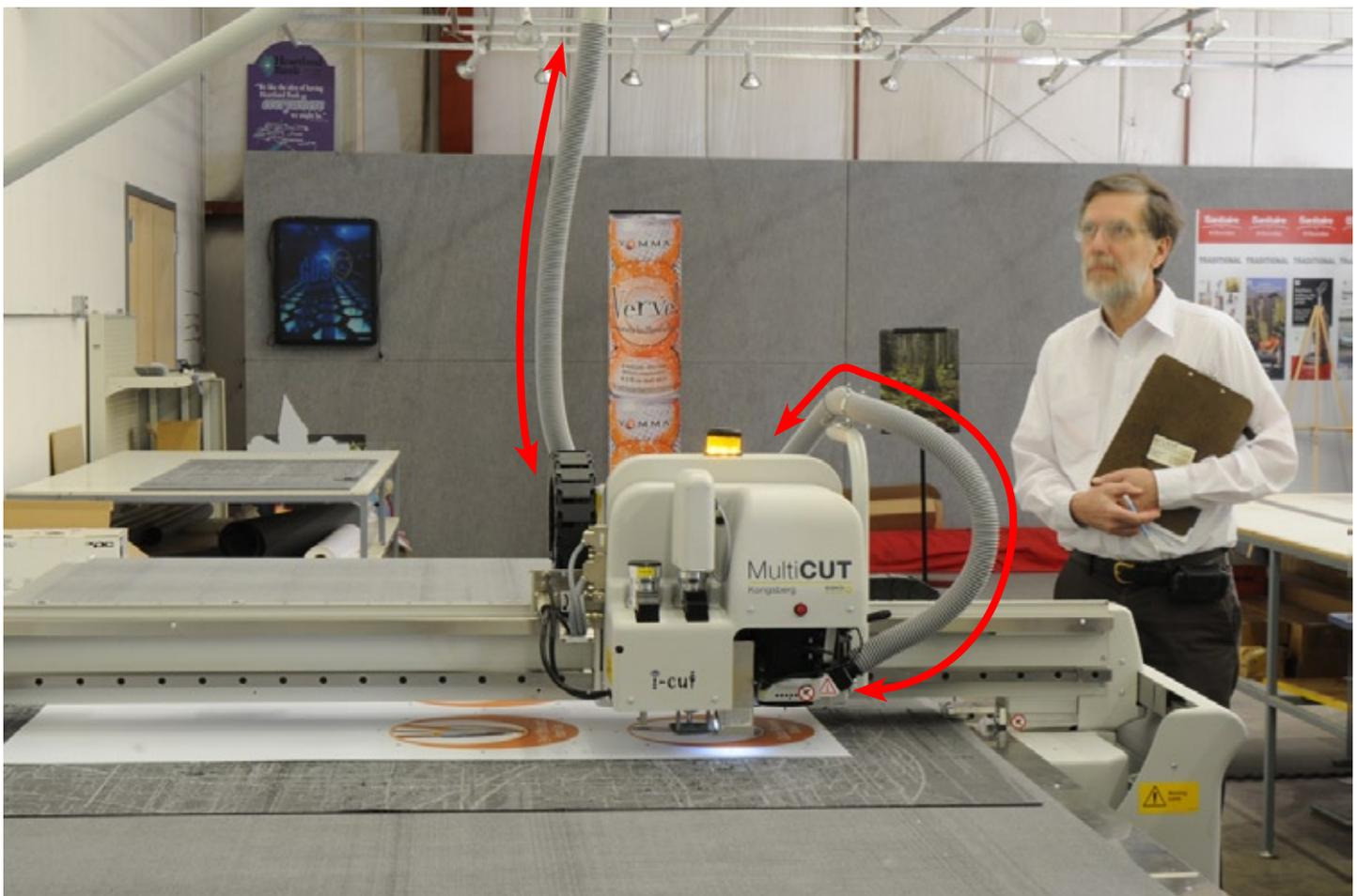
*The cutter has a suction hose with a vacuum cleaner to reduce the dust and detritus of the material that is being cut.*
