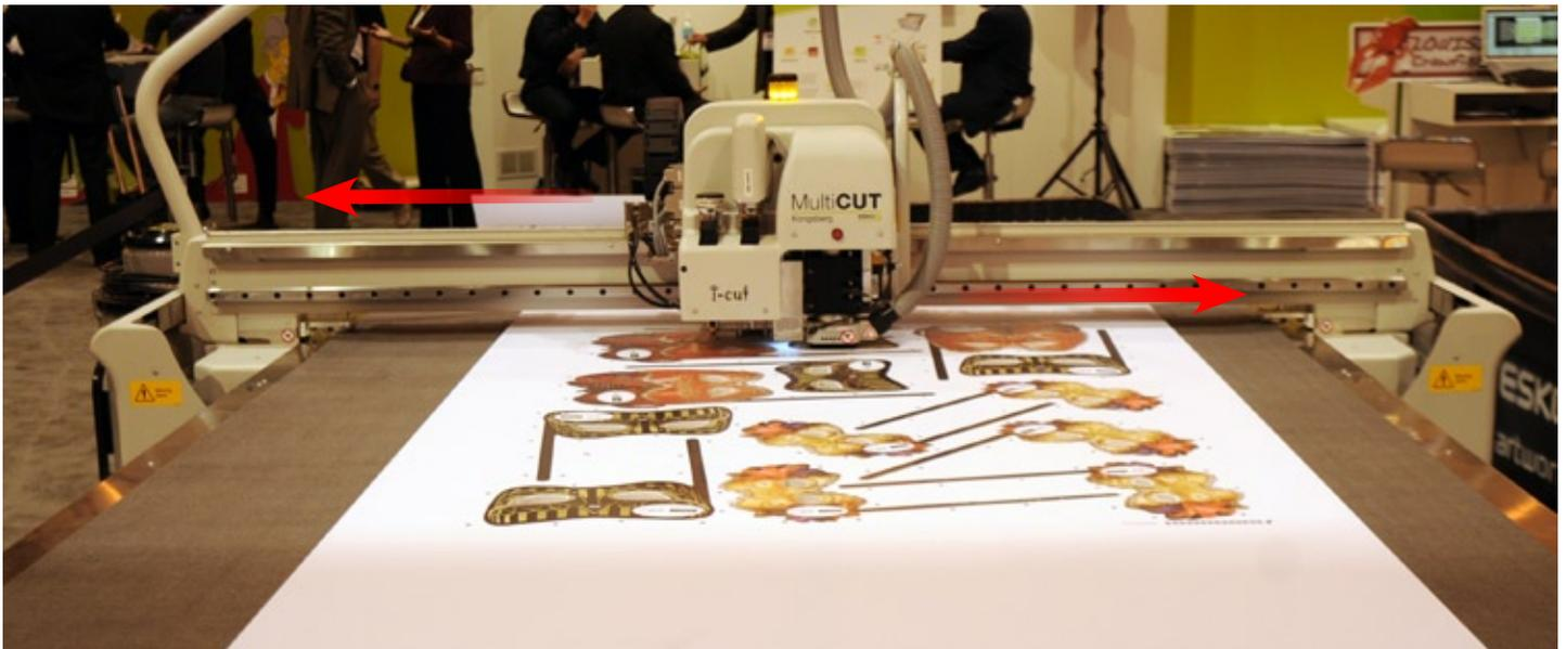
The Kongsberg XL cutter series uses appropriate brushless servo motors. The advantage of using a servo motor is that it provides feedback and can correct its positioning.
