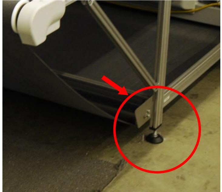
There are six leveling supports on the XP cutter that I inspected at VISCOM Paris 2009.
