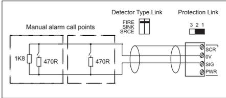
Figure 2.11 Connections for manual alarm call points
