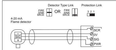
Figure 2.14 Connections for 4-20 mA 3 wire Flame detector
