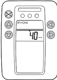
Figure 3.2 User display Gasmaster 1
