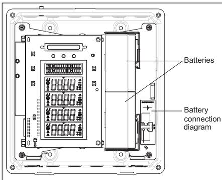
Figure 4.1 Battery replacement
