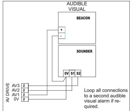
Figure 2.16 Connections for AV drive
