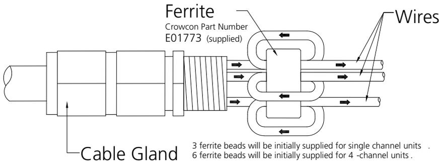
At minimum, the following cables require this application: Mains Power, Channel Input, and Audible Visual Alarm
