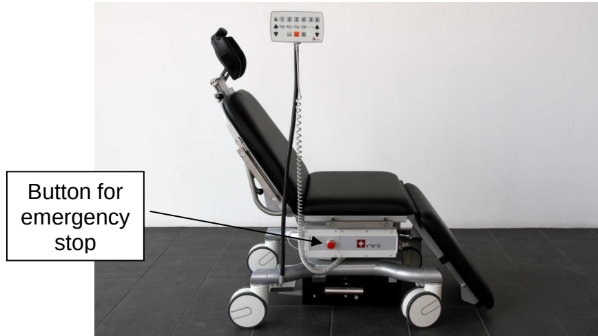
Location of button for emergency stop
