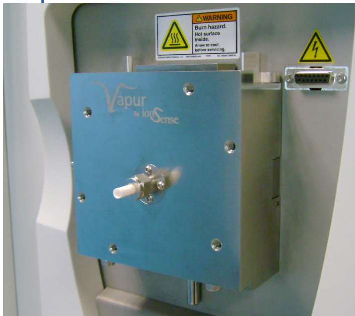
Figure 7: Vapur interface attached to Thermo Ion Max
