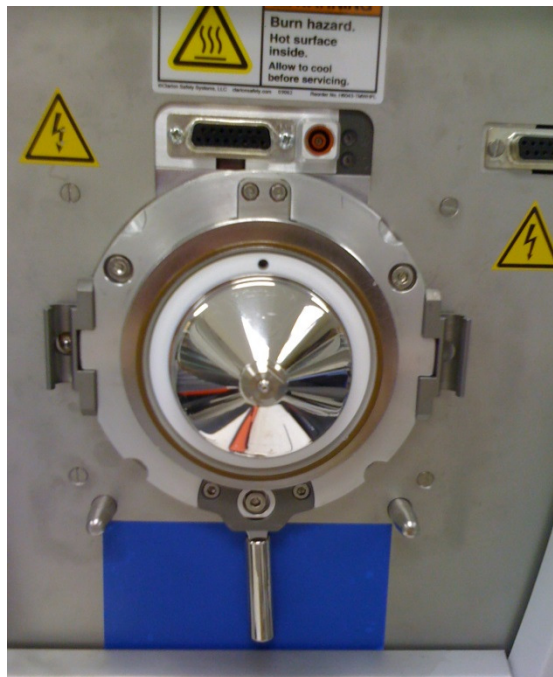
Figure 4: source region with the Thermo ion sweep cone removed
