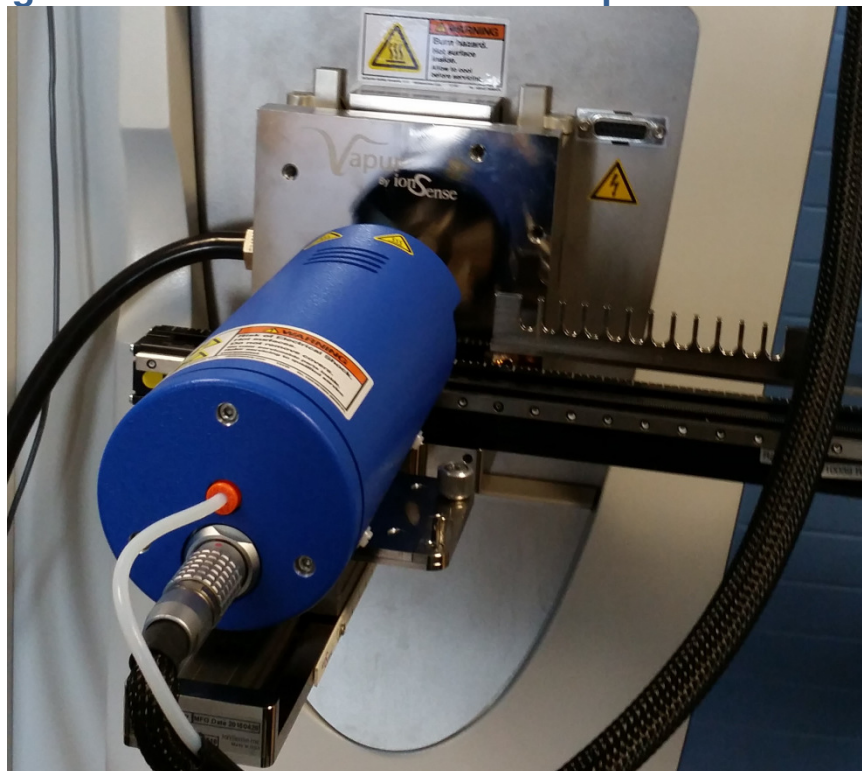
Figure 11: DART SVP source attached to Vapur Interface
