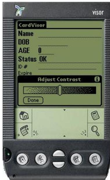
Adjust the contrast by using the stylus to “grab” the slider bar on the contrast pop up.
