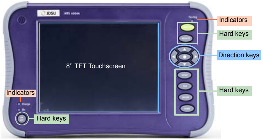
Fig. 3 6000A V2 Platform - Front Panel description
