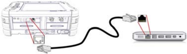
Fig. 34 Connection 6000A V2 Platform and PC
