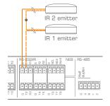
When used as dual IR port: Connect the IR 1 emitter to e.g. T1 (white striped wire) and black wire on IR 1 emitter to IR 2 emitter (white striped wire), and black wire from IR 2 emitter to GND, as shown here above.
