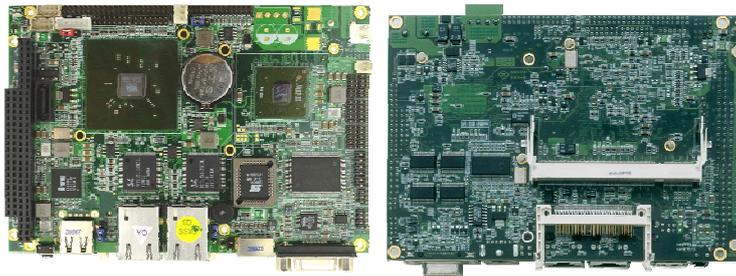
The HS-2615 is a VIA CX700(M) chipset-based board designed. The HS-2615 is an ideal all-in-one embedded engine board. Additional features include an enhanced I/O with CF, 8-bit I/O, CRT/LVDS, TV-Out, dual LAN, audio, SATA, 4 COM, 6 USB2.0, and PC/104 interfaces.
