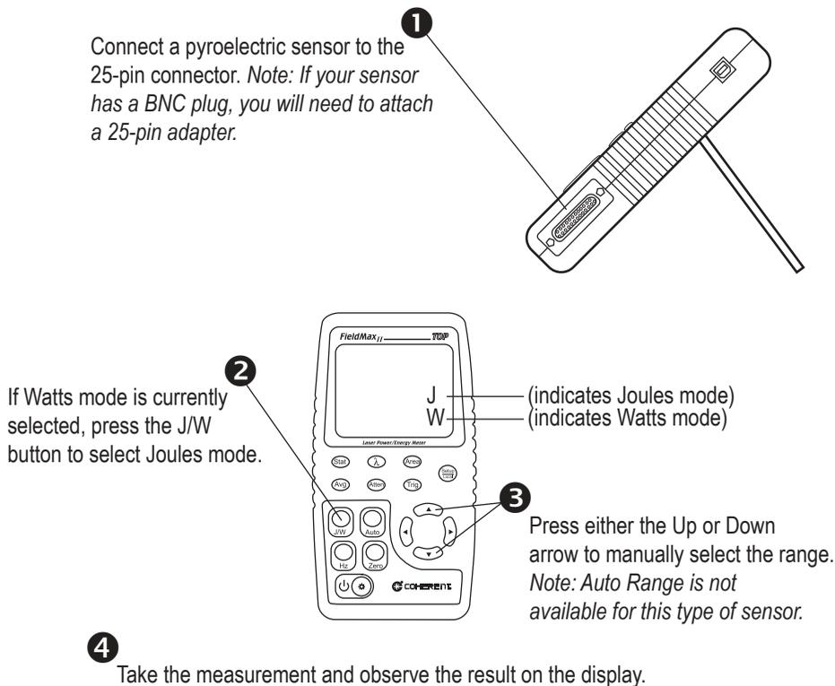
**Figure 3. Measuring Energy With a Pyroelectric Sensor**
