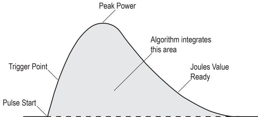
**Figure 17. Measuring Energy - Pulsed Thermopile Joules Mode**
