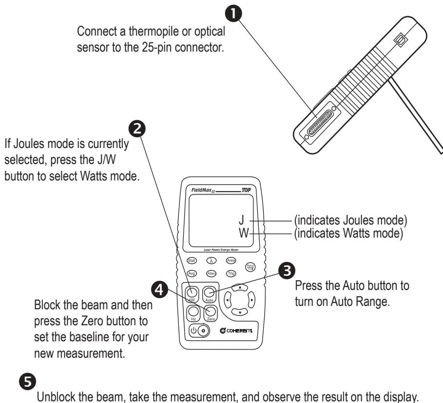
**Figure 2. Measuring Power With a Thermopile or Optical Sensor**
