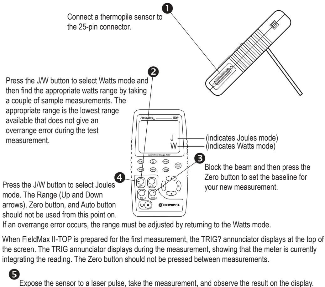
**Figure 4. Measuring Energy With a Thermopile Sensor**
