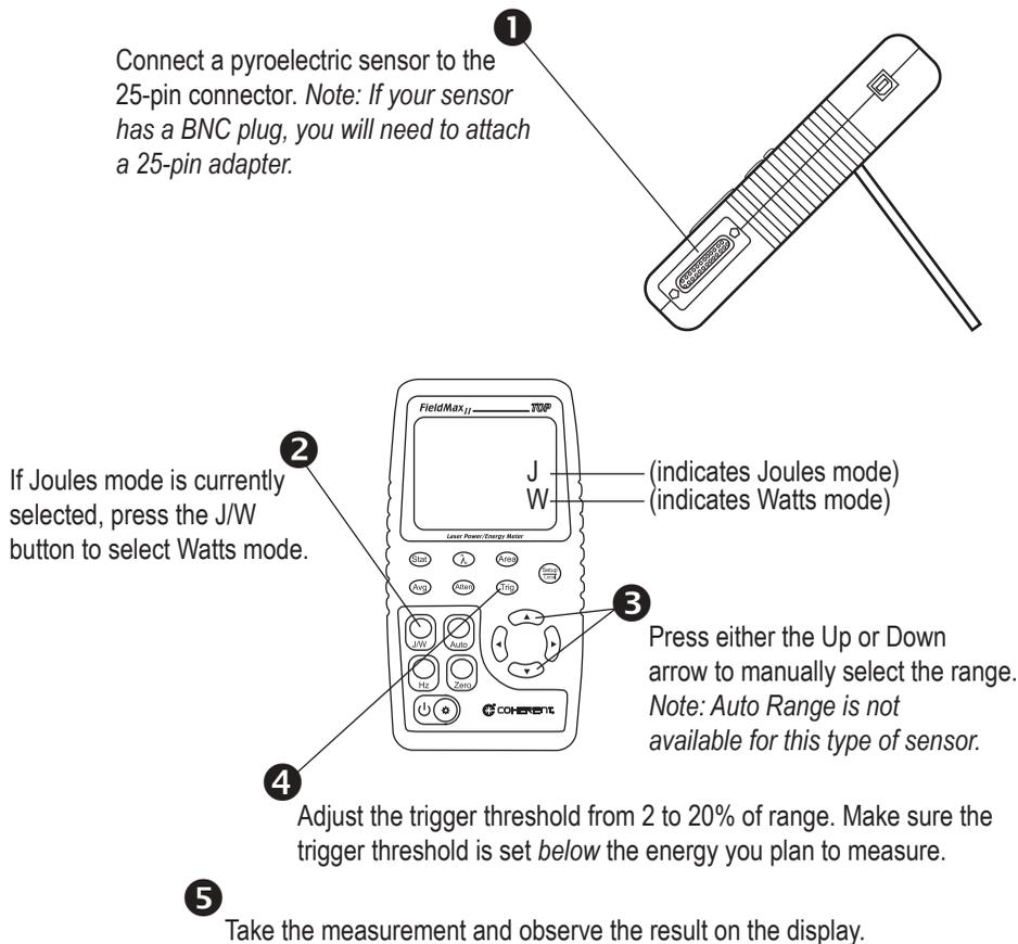
**Figure 1. Measuring Average Power With a Pyroelectric Sensor**
