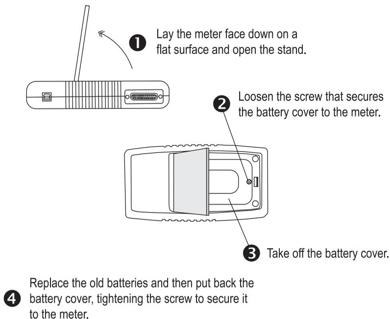
**Figure 9. Battery Replacement**
