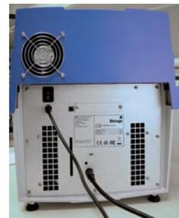
*The instrument shall be connected to properly grounded mains outlets using the supplied power supplies; see the Installation and Safety document.*
