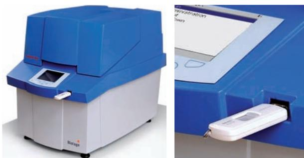
Run files are transferred to the instrument using the USB memory sticks supplied with the system.
