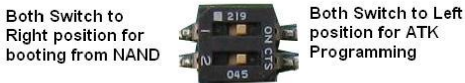
Figure 5: Switch Position for Boot Strap Mode
