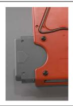
Insert the Self-diagnosis Module into the suitable slot. Push gently until you hear it click into place; the retaining tab will lock the self-diagnosis module into place in its slot.
