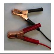
Connect the power supply clamps to the vehicle battery; be sure to connect the red clamp to the positive terminal and the black clamp to the negative terminal and make sure that the green light is flashing.
