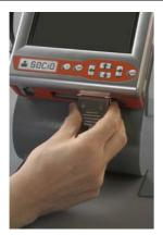
Connect the diagnostic cable connector to the connector of the self-diagnosis module (BBAD). If the connector has been inserted correctly, you will hear the retaining clip click into place, indicating the connector has locked into place in the mating piece.
