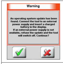
Follow the on-screen instructions, ensure the tool is powered from the outside and (if available) insert a charged battery.
