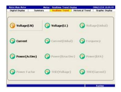
PM1600 can display various power values including voltage, current, power factor...etc. alone the time for each meter. The displayed item for each meter is varied according to the setting in the configuration mode (see chapter 6.2.4). Auto scale is the default for trend display. User can modify Y-axis scale by using Y maximum and minimum button.
