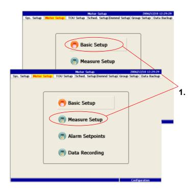
Use the up/down Arrow key → to navigate among the functions, then press the Enter key
