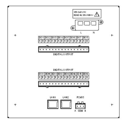
LAN1: To connect with Transducers over Ethernet network LAN2: To connect with PC for web server function
