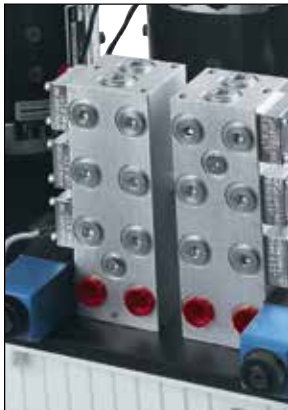
Attached manifold on Hydro 2 HPU
