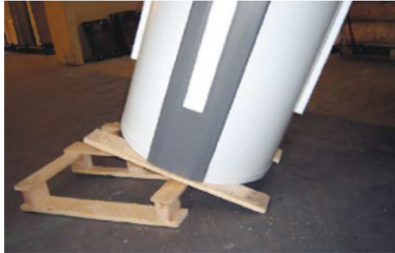
4. Removal of product : a: Glide product carefully to one side a bit. b: Bow over to the same side together with 2 pcs. of wood beneath.
