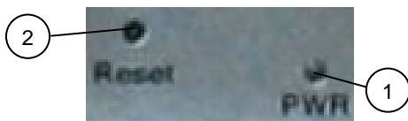
Fig. 18: M@CII 70/104/121/150 detail for Power LED and Reset button on the bottom (rear) side
