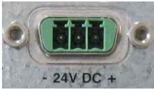
Fig. 17: Detail: DC Power connector at the bottom (rear) side of the M@CII 70/104/121/150 system
