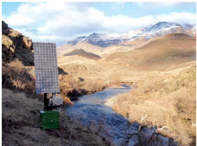
A PIT system on the Imnaha River, Oregon, where a hybrid thermoelectric generator (TEG) is in use that utilizes solar power to help reduce fuel consumption.
