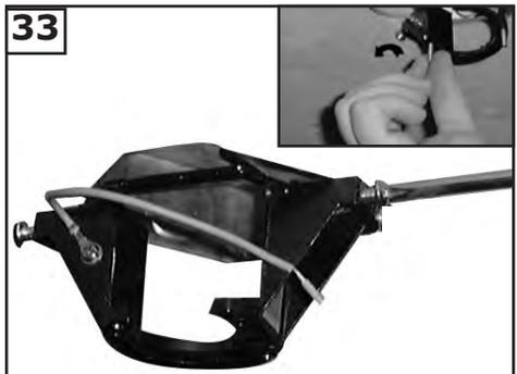
**33** Install two screws corresponding with the "L" shaped holes in the canopy only part way so that canopy can twist into place. Remove the all thread studs from the lower part of the mounting bracket.
