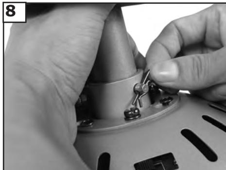
Insert downrod into yoke on top of the Fan Body. Align the hole in the Downrod with the hole in the Yoke. Insert the Pin through the Yoke and Downrod until the point appears on the other side. Install the keeper to pin.
