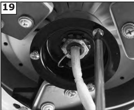
**19** Loosen 2 screws with key slots and remove 1 screw without slot from motor plate and save screw.
