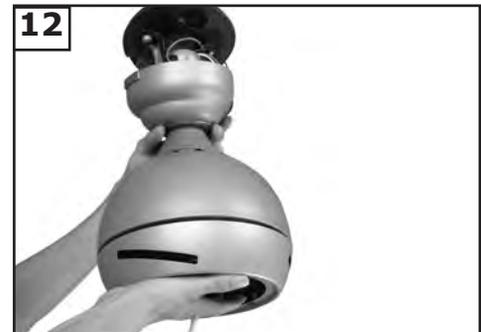
**12** Hang assembled fan from the mounting bracket installed to ceiling in previous step. Make sure the fan is hanging straight. Rotate fan until the tab on the Mounting bracket engages the slot on the Downrod Ball. This must be done to prevent the fan body from rotating when the blades are in motion.
