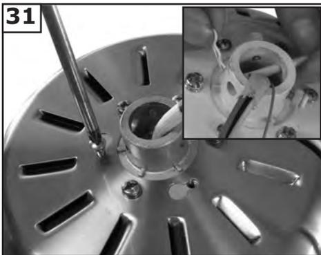
**31** Remove 2 screws in yoke and keep them then cross pin (see insert). Remove 3 screws with keyhole slots from top of fan.
