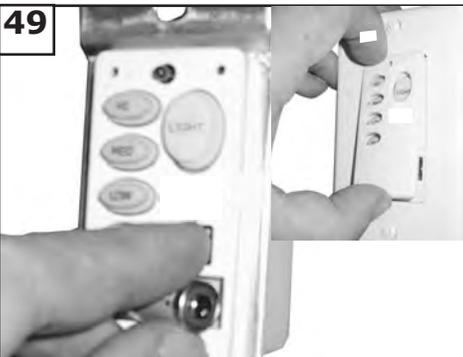
49 Remove cover by snapping off from top or bottom. Install 12V battery into wall remote. Duracell MN21/Eveready A23/GP 23A all 12V
