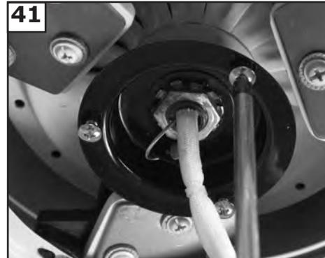
**41** Loosen 2 screws with key slots and remove 1 screw without slot from motor plate and save screw.
