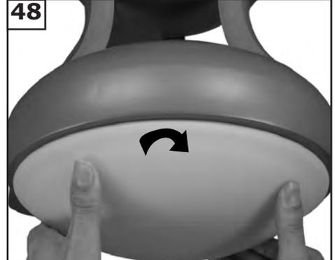
48 Attach glass by locating dimples in light fixture with the grooves in glass and twisting clockwise till tight.
