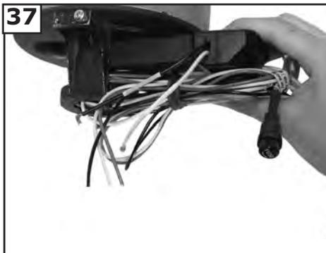
**37** Slide remote receiver into mounting bracket.
