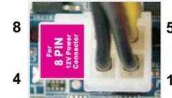
4-pin 12V ATX power supply installation
