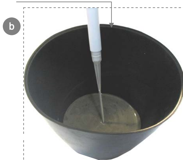
Aspirate 6.5 - 7.5 \mu l of the mixture
