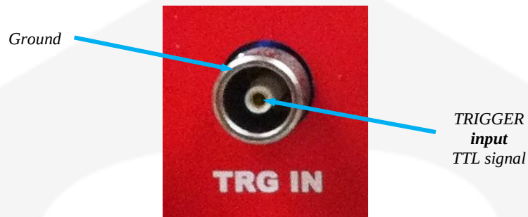
Figure 5 – Trigger input connector
