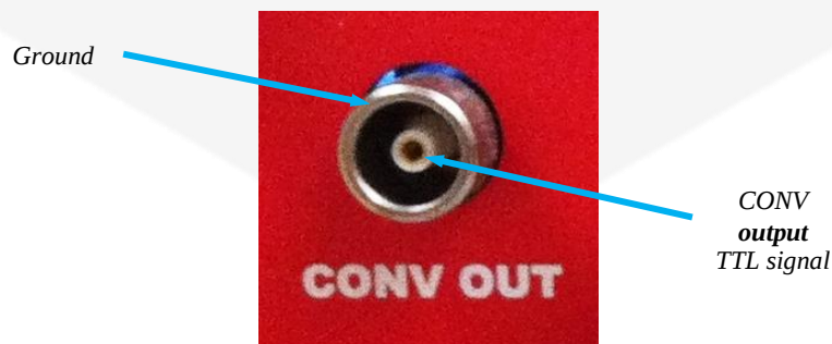
Figure 6 – CONV output connector
