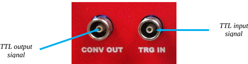
Figure 4 - I/O Interface Connector
