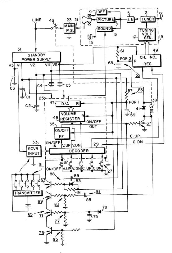
SHORT-TERM POWER DROPOUT ARRANGEMENT USEFUL IN A TELEVISION RECEIVER
