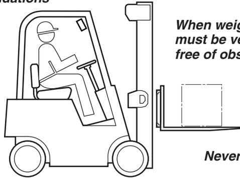
**When weighing load, mast must be vertical and load is free of obstacles**
