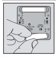
[3] Insert the batteries with the + and – poles facing the correct direction.
