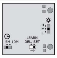
[6] Slide the "LEARN" switch to "SET". To confirm, the receiver switches on and off two times.
