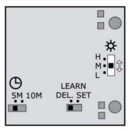
[4] Set the light sensitivity switch to "M" or "L". "M": Sensor works in areas with little light or in the afternoon (15 to 25 Lux). "L": Sensor works in dark areas or late in the evening (0 to 15 Lux).
