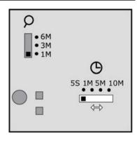
[8] Set the time for switching off. As soon as no more movement is detected, the transmitter will automatically send an "off" signal after 5 seconds, 1 minute, 5 minutes or 10 minutes.
