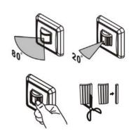
[10] The detection range is maximum  $80^\circ$  and minimum  $20^\circ.$  Remove or reposition the screens to adjust the angle.
