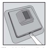
[1] Remove the front with the sensor and the wall plate from the base.
