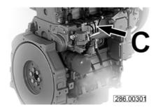
The engine's type plate comprises the engine model and serial number.
