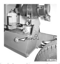
When checking the oil level, the machine must be on level ground with the tools lowered, and the oil must be cool.
