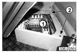
The switch board, relays and fuses (1) are located underneath the driver's seat.
