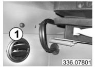
The internal circulation vent (1) is located to the right of the driver's leg. Keep the vent normally closed. If you wish to heat the cabin quickly, open the vent so that the same indoor air is recirculated through the heater and the cabin heating improves.
