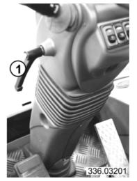
Adjust the tilt angle of the steering column by loosening the locking lever (1) on its left side so that the steering column controls are at a convenient distance and you can maintain an ergonomic driving position together with the seat adjustments.
