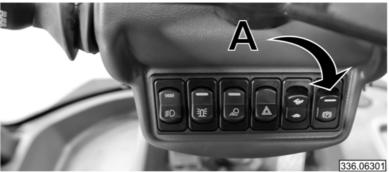
The machine must stay safely in position on a slope of 20% when the parking brake is engaged (switch A is ON).
