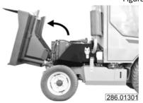
The bonnet/platform body can be tipped by opening the latch (A) and turning it as shown in the figure. Always ensure that the bonnet is tipped to its extreme position, if you are working underneath it.
