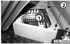
The switchboard (1), fuses and relays are located underneath the driver's seat.
