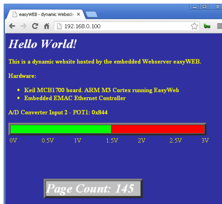
Figure 12 Webpage that shows the value of the ADC value of the MCB1700 board.
