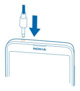
Do not connect products that create an output signal, as this may damage the device. Do not connect any voltage source to the audio connector. If you connect an external device or headset, other than those approved for use with this device, to the audio connector, pay special attention to volume levels.
