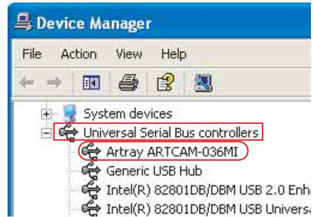
If installing device drive is succeed, model name is shown under the device manager.
