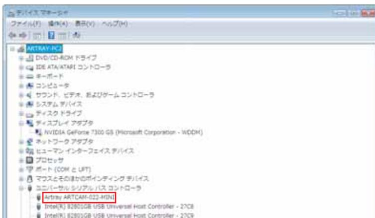
Check if camera name 「Artray ARTCAM-022-MINI」 is shown under the Universal Serial Controller (USB) tree.
