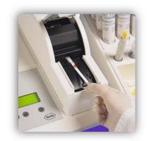
When the strip is inserted correctly PLEASE CLOSE LID will appear on the display. Close the lid.
